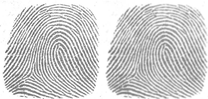
Fig. 5. An image acquired using our sensor (left), Diffused fingerprint image itr. = 3, \lambda = 0.125 , neighborhood = 8 (right).
