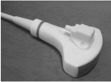
Figure 1: The electromagnetic sensor is attached to the transducer.
